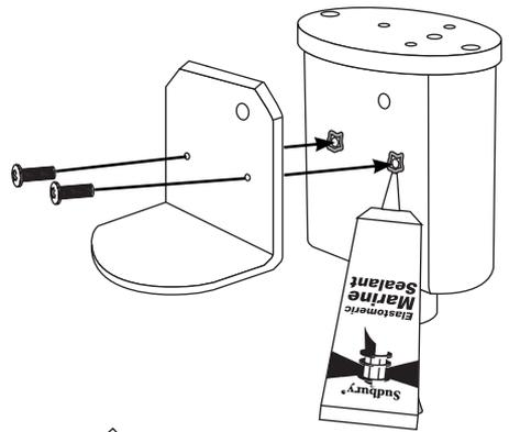
**6** Using marine adhesive sealant apply some around the two holes and perimeter of the top as shown.
