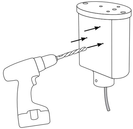
**5** Using the hardware that came with your light, secure lights to the front and back of the LTB-BOX or LTB-BOXW.
