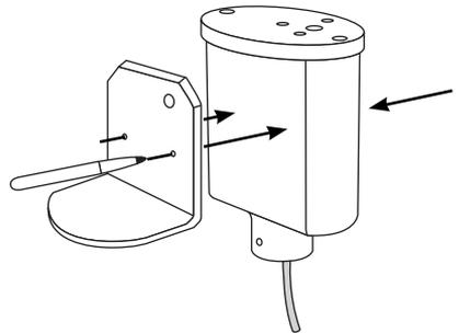
**4** Using a drill bit drill the holes you just previously marked on both sides.
