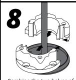
Combine the two halves of the plastic base and mount onto rubber base gasket. Be sure to stagger the seams as shown by the two black arrows.
