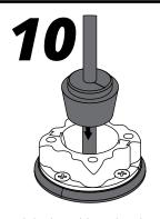
Slide the rubber plug down into the plastic base.
