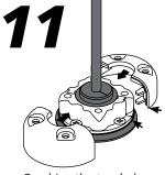
Combine the two halves of the outer shell. Be sure to stagger the seams as shown by the two black arrows.
