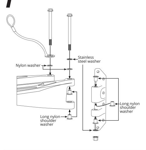
Please note that when installing the Seaview Mast Mount, have it facing the forward end of the boat.
