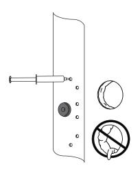
Insert the black nylon shoulder washers into the correct holes on the mast mount feet. Use the supplied rivets to secure the mast mount to the mast.
