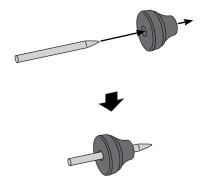
Insert the rubber grommet into the hole you drilled for the cables.
