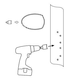
Punch a hole through the rubber grommet using a sharp dowel.
