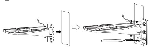
Using a 3/16" drill bit, drill all the marked holes.
