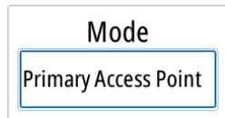
Only one WIFI-1 may operate as 'Primary', which determines that the device is acting as DHCP server. Only one DHCP server may exist on a network at a time.
