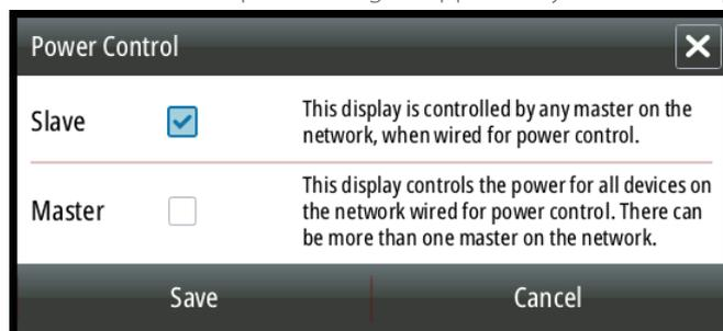
Set to 'Slave' if the yellow wire is connected to ignition or to a stand-alone switch that applies 12V/24V. Set to Master to make this device turn on other devices when powered up.
