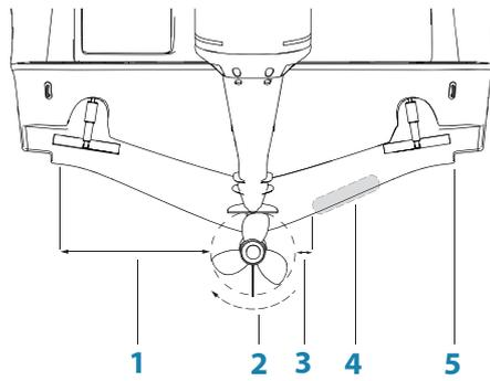
**1 Avoid mounting within 1m (3.3') to port of propeller**
